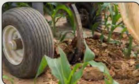
Shovels help lift up the edges of plastic. Gauge wheels determine the depth of the coulters and shovels.
